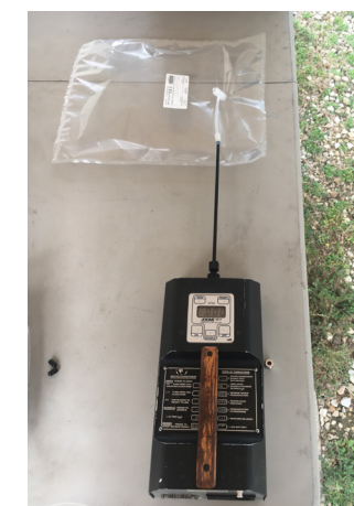
Analyzing field sample using a Jerome 631-X
