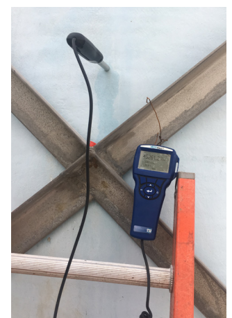
Analyzing discharge flow rate using a TSI VelociCalc 9545
